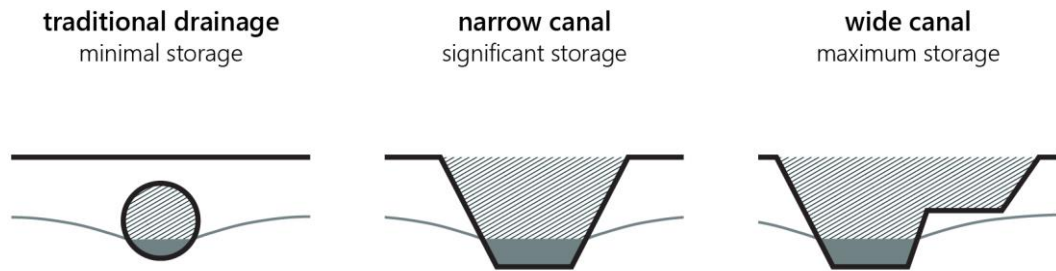
Figure 4.3: Illustration of creating extra storage capacity when replacing pipes with surface storage and drainage.
