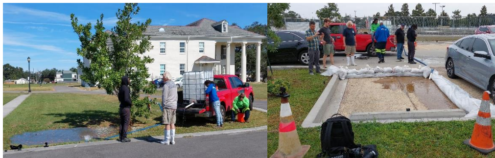
Figure 6.3 left: full-scale test at raingarden Milne (test number 14, table 1). Right: full-scale test at permeable pavement after building a confined space with plastic and sandbags.
