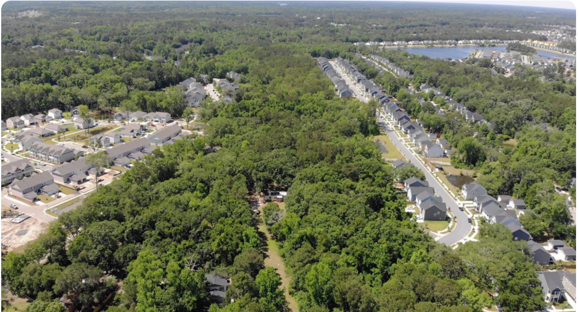
An aerial image of the Barberry Woods neighborhood on Johns Island, SC. WK Dickson's design rerouted water through the central tree-covered area to reduce flooding in the neighborhood. (Photo by WK Dickson)
